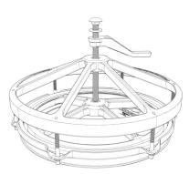
Turn the long carriage bolt clockwise until it makes contact with the bottom insert.
